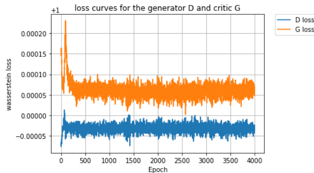
Figure 8: Loss curves for WGAN with the best grid search parameters: n\_critic=5 and batch size=32.
